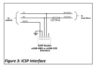
It is recommended that the uDRIVE module be socketed on the application board so that it can be easily removed for PmmC programming. If the module is to be permanantly fixed and cannot be removed then access must be provided for PmmC
