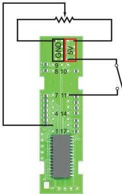
Typical Digital Input Wiring
